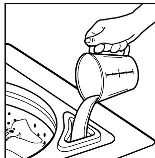
**bleach** into the liquid chlorine bleach dispenser. Bleach will be diluted automatically during the wash part of the cycle.
