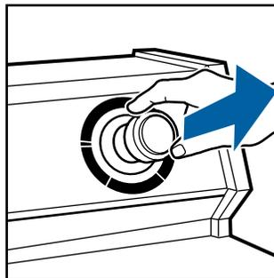
**NOTE:** To **stop** the washer at any time, push in the Cycle Control Knob. To **restart** the washer, close the lid (if open) and pull out the Cycle Control Knob.
